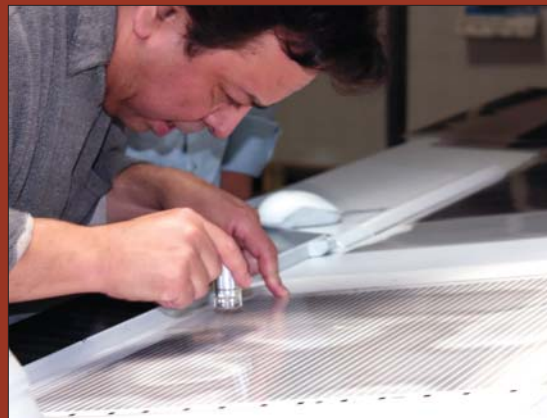
The pitch test requires a careful look at the test sheet to calculate the proper interlace of the final product.
